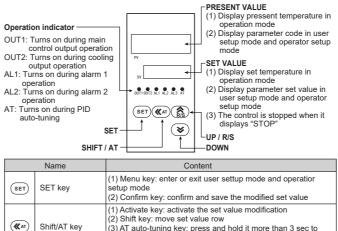
3) AT auto-tuning key: press and hold it more than 3 sec to start or exit auto-tuning (1) Up key: increase set value, move among parameter menus 2) R/S: in operation mode, press and hold it more than 3 sec Up key/ R/S to change between RUN and STOP operation mode Decrease set value, move among parameter menus Solution (Section 2017) Down key
